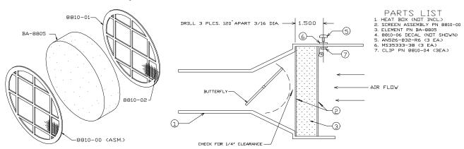
NOTE: After initial installation of filter assembly, fill out FAA form 337 for return to service. On future replacement of parts this form will not be required.
