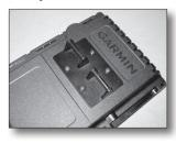
Using the four supplied 6-32 black screws, attach the bracket to the back of your GPS. Tight securely making sure to not overtighten the screws - it may result in cracking of the bracket.
