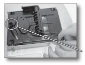
The bolts we provide have an integral washer on the screw-head side. This provides adequate distribution of force on the plastic to keep it from cracking. Position the hard-ware so that the screw head is located on the plastic side and the nut is on the outer side of the metal rail. Please, be sure not to overtighten the screws, it may result in cracking of the plastic of the Panel Dock.
